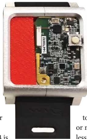
4. QuickLogic's TAG-N module uses the Nordic Semiconductor's nRF51822 Bluetooth Smart and the Articom S2 smart sensor hub.
